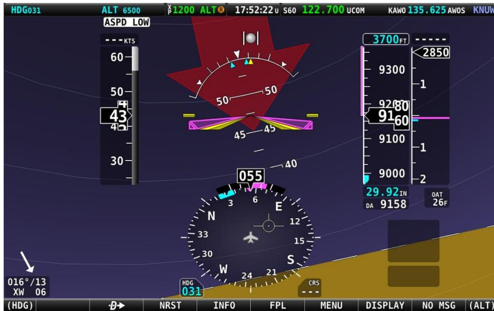
Figure 74 – Extreme Pitch Warning Indicator Arrows
