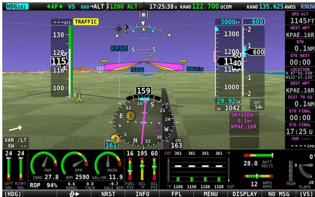
Figure 69 – SkyView HDX Synthetic Vision Traffic Alert
