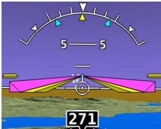
Figure 233 – Single Cue / Inverted-V with Autopilot Servos Engaged
