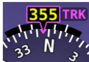
**Figure 41 – GPS Track substitute for Magnetic Heading**
