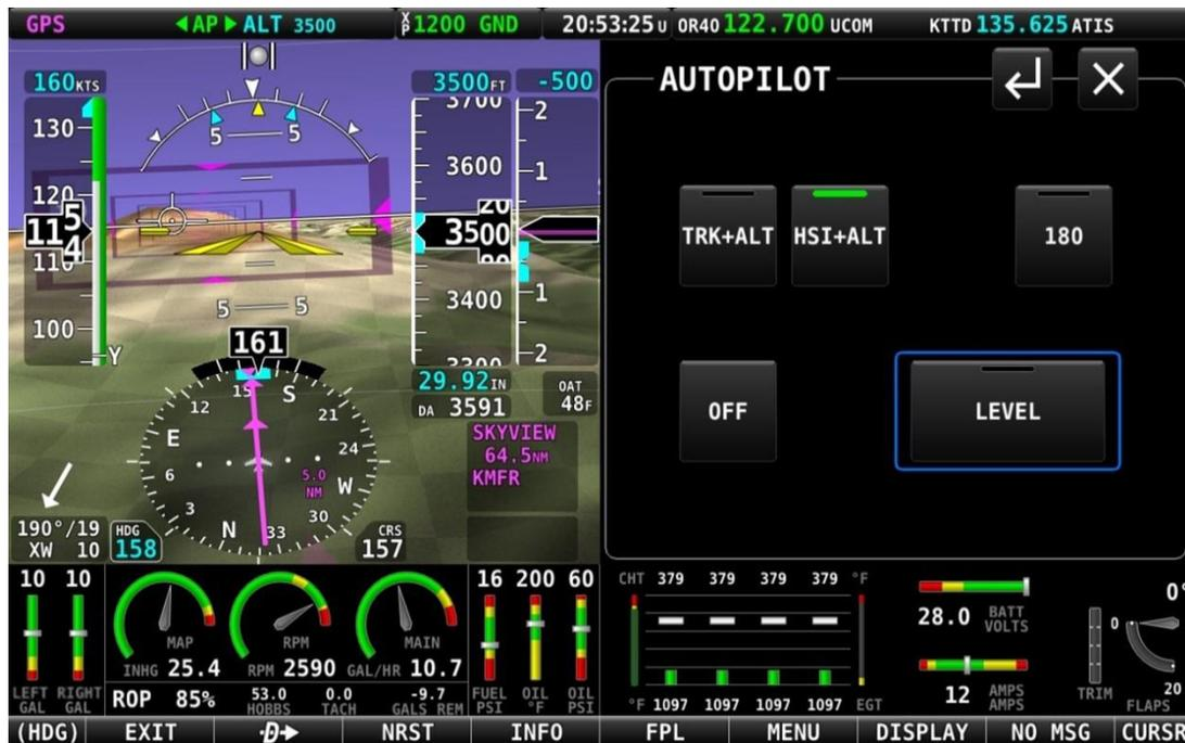
Figure 226 – HSI+ALT mode is engaged
