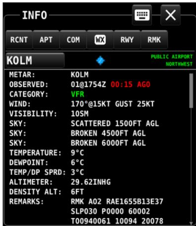
Figure 187 – METAR – Decoded
