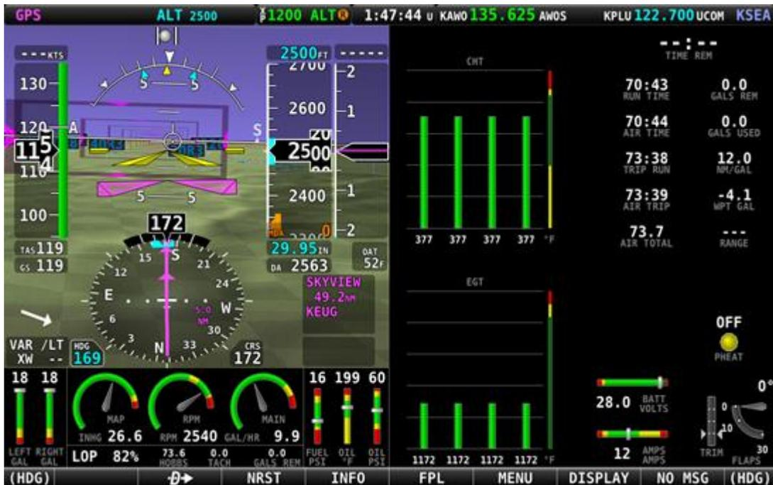
Figure 15 – 50% PFD / 50% ENGINE with ENGINE BOTTOM BAND
