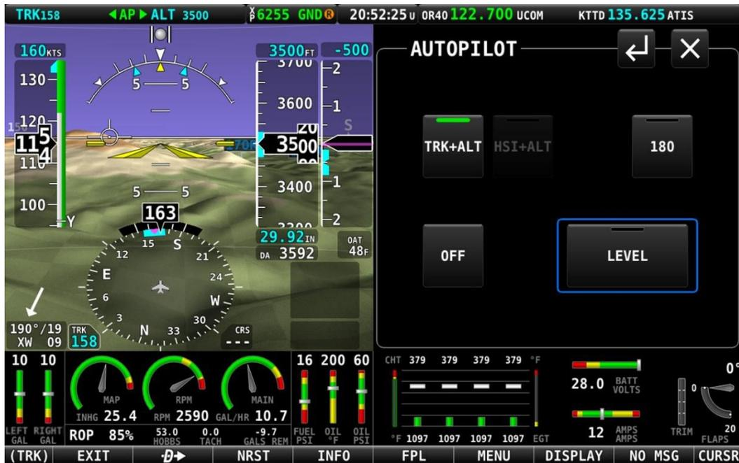
Figure 225 – TRK+ALT mode is engaged
