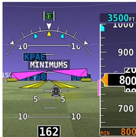
Figure 37 – MIN Bug and “MINIMUMS” Alert
