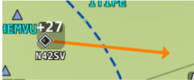
Figure 122 – Traffic Targets Display of Tail Numbers
