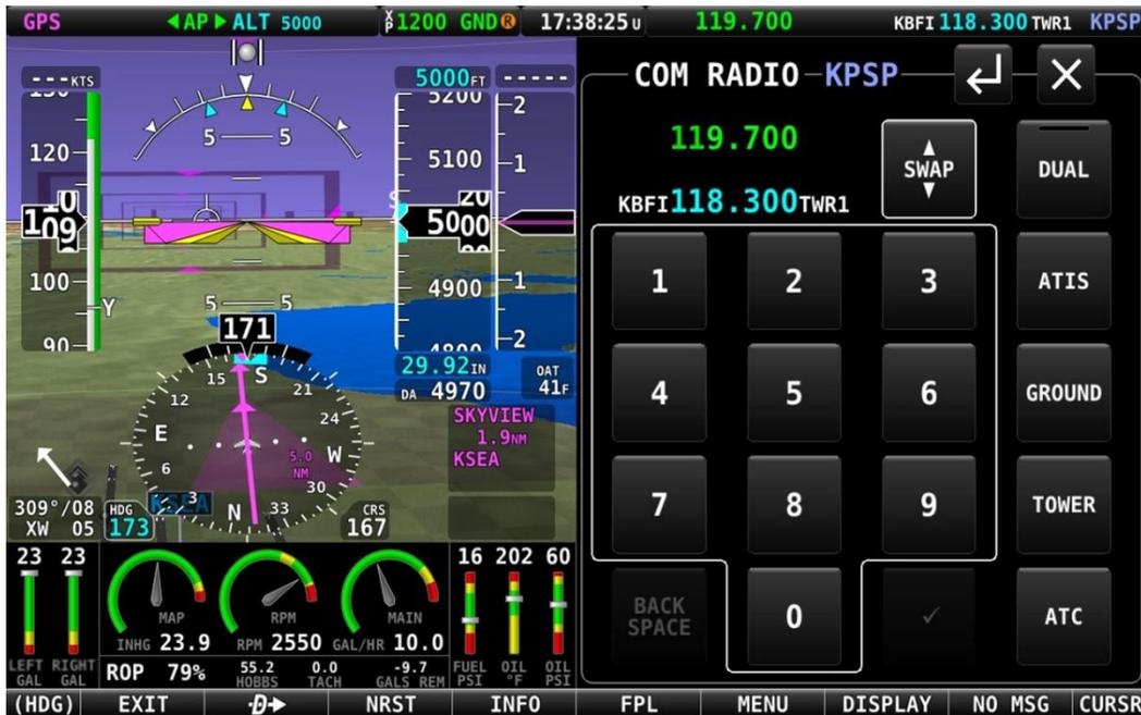
Figure 242 – Com Radio Control Panel
