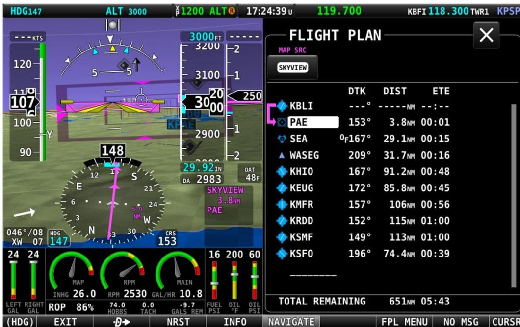
Figure 154 – Active Flight Plan: Flight Plan shown
