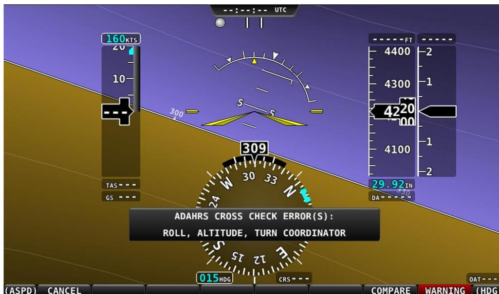
Figure 87 – ADAHRS Cross-Checking Disagreement
