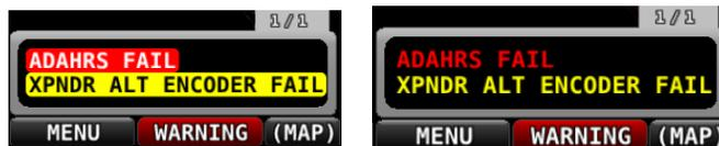
**Figure 253 – Unacknowledged (left) and Acknowledged (right) Alarms**
