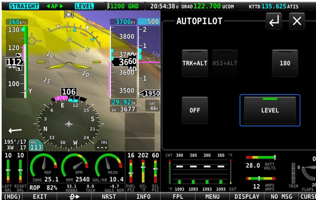
Figure 228 – LEVEL mode is engaged
