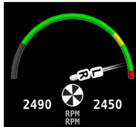
Figure 201 – Example of a Synchroscope and a Combined RPM Widget
