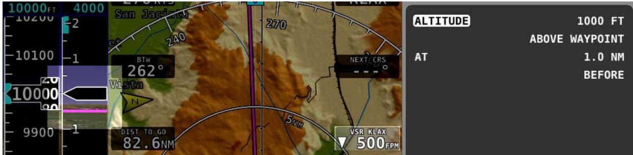
Figure 39 – Vertical Speed Required to Destination
