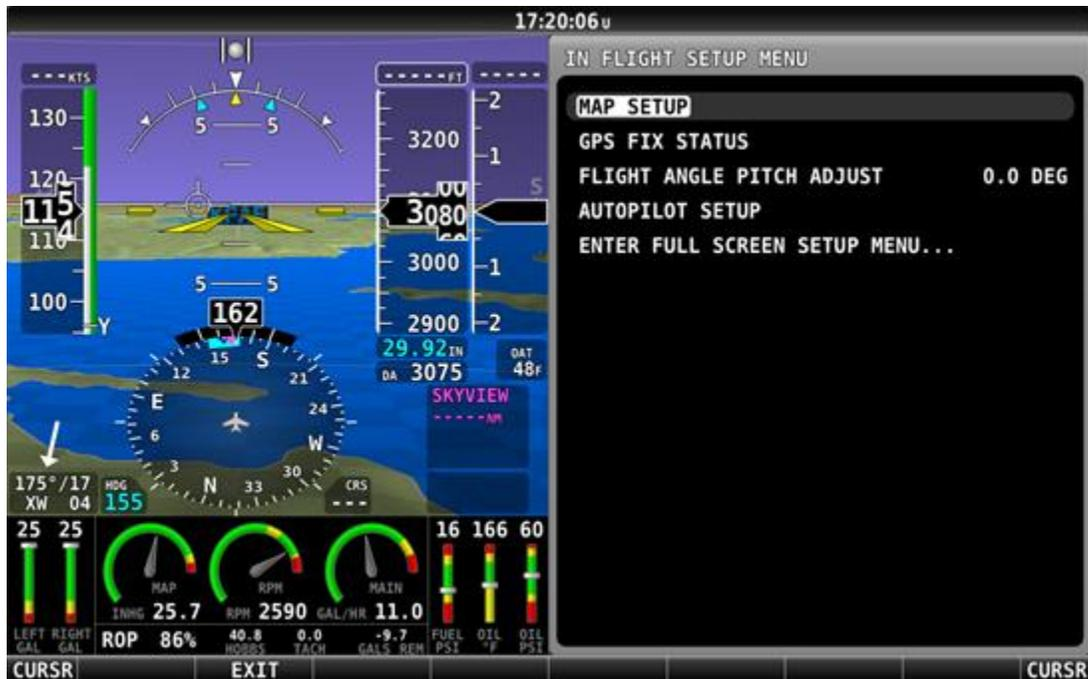
Figure 26 – IN FLIGHT SETUP MENU
